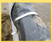
Film clamping by spring construction. After the silage, easily to be removed from the upper side.
